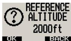
Adjust the reference altitude using the rotary control. This is the altitude that the pilot wants to maintain. Press the F1 key to accept, press the F2 key to return to the main display.
