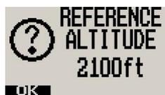
Enter the reference altitude you would like to use in relative mode. Use the rotary control to adjust the reference altitude. Press the F1/up key to accept.
