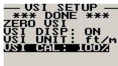
This is a function that is used to calibrate your VSI to read exact rates of climb or decent. This function works as a percentage of initial reading. The default setting for this function is 100%. Increasing this value increases the VSI reading and decreasing the value decreases the reading.
