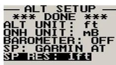
Select the resolution of the output data, a selection of 1,10,25 or 100 ft can be made.
