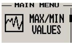
To avoid false recordings, the maximum values function is only activated 10 seconds after the instrument has powered up.
