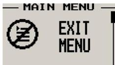
Pressing the rotary control on this menu item will cause the ALT-2 to exit the menu system. All changes made during navigation of the menu system will be saved in non-volatile memory on exiting the menu system. If you remove power before exiting the menu the instrument will not save any changes.
