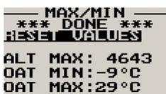
Move the highlight over this menu item and press the rotary button to reset the maximum altitude and airspeed values to the current values.
