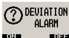
Select whether you want the altitude deviation feature enabled or not. Press the F1 key to enable the altitude deviation feature, press the F2 key to disable the altitude deviation feature.
