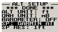
Select the protocol of the RS232 output message. The protocol can be selected between GARMIN AT, Magellan, Northstar/Garmin, Trimble/Garmin, MGL Avionics and Microair UAV. Please see section 5 for more information.
