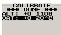
The ALT-2 is calibrated in degrees Celcius. The ALT-2 is calibrated at the factory using a precision laboratory thermometer. If recalibration is required then adjust the value using the up/down keys or the rotary control until the temperature matches the reference ambient temperature.
